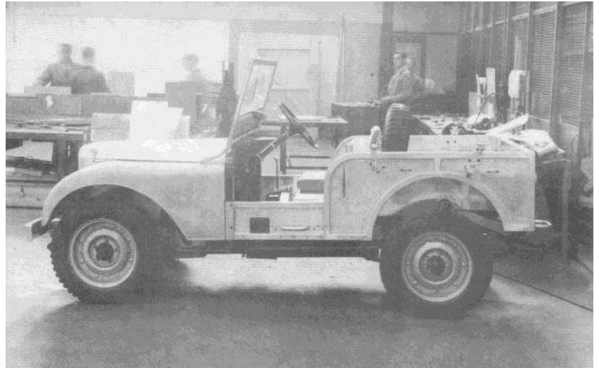
Earliest known picture of the Centre Steer Prototype, taken in the Rover Jig Shop on the 30th of September 1947
