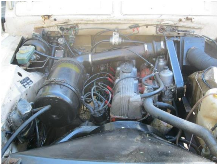
R6 engine installation in a Land Rover
