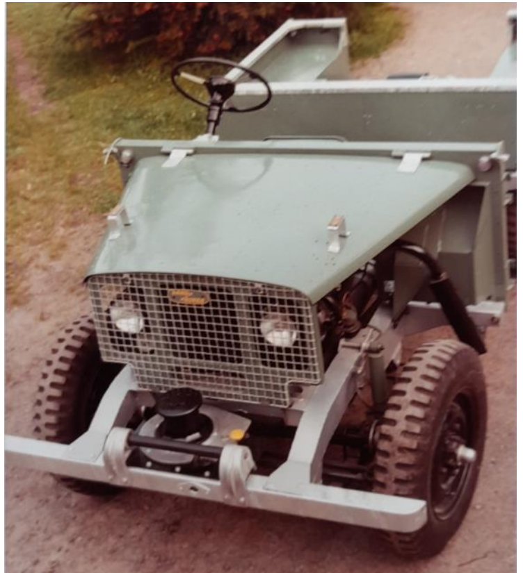
Capstan and guide roller mounted
