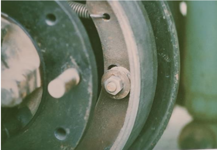
The automatic brake adjustor assembly in place
