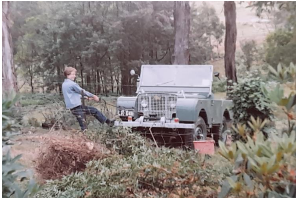
The capstan winch at work
