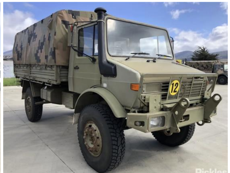
12/1986 Mercedes Benz Unimog U1700L cargo, showing 91,490 km's, OM352A turbo diesel engine, 8 x Forward Gears, 8 x Reverse Gears, $33,750.
