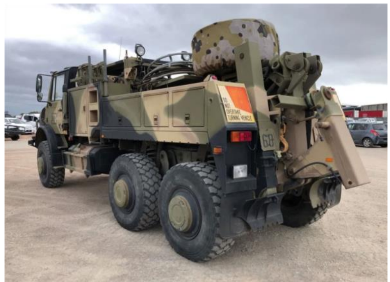
2000 Mercedes Benz U2450L Unimog, 6 x 6, medium wrecker, showing 14 km's, 1714 engine hrs, log book, 5958cc 6-cyl turbo-charged intercooled OM 366 LA diesel engine, 177 kw @ 2600 rpm, 16 spd manual gearbox (in fwd & rev), part-time 6x6, diff' locks, portal axles with hub-reduction, disc brakes, driver operated central tyre inflation system, air conditioning, fitted with 1998 Palfinger P067 Crane, hydraulic under-lift towing system, multiple side storage units, front winch, rear work lights, main boom, May be incomplete and non-operational. As is, where is with faults, if any. No warranty or guarantee. Inspection is advised. $150,500.
