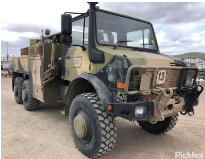
2000 Mercedes Benz U2450L Unimog, 6 x 6, medium wrecker, showing 14 km's, 1714 engine hrs, log book, 5958cc 6-cyl turbo-charged intercooled OM 366 LA diesel engine, 177 kw @ 2600 rpm, 16 spd manual gearbox (in fwd & rev), part-time 6x6, diff' locks, portal axles with hub-reduction, disc brakes, driver operated central tyre inflation system, air conditioning, fitted with 1998 Palfinger P067 Crane, hydraulic under-lift towing system, multiple side storage units, front winch, rear work lights, main boom, May be incomplete and non-operational. As is, where is with faults, if any. No warranty or guarantee. Inspection is advised. $150,500.
