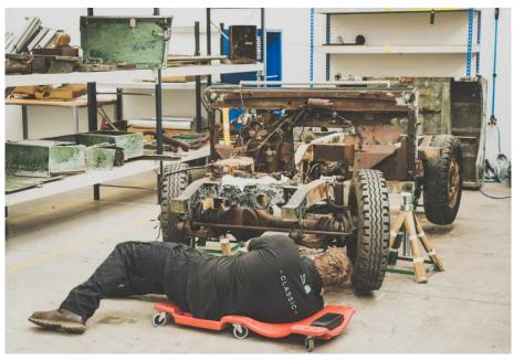
and tireless passion of the experts at our Classic Works facility." said Calum McKechnie, Head of Land Rover Classic. While the front axle required no significant repairs, the rear axle showed signs of extreme damage and fatigue. To understand the extent of the problem, the original part was X-rayed and depth-tested using state-of-the-art techniques and found to
