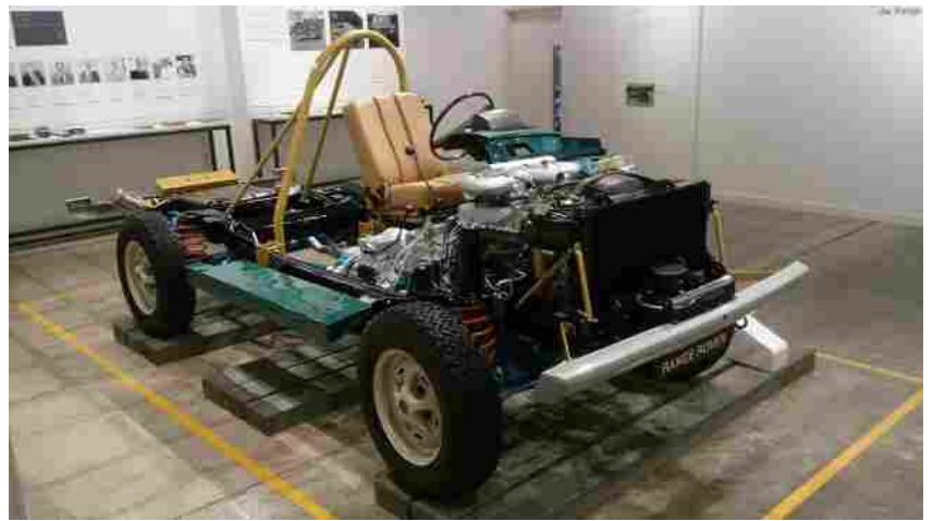
The fully driveable 1970 cutaway Range Rover engineering model designed to show the inner workings.
