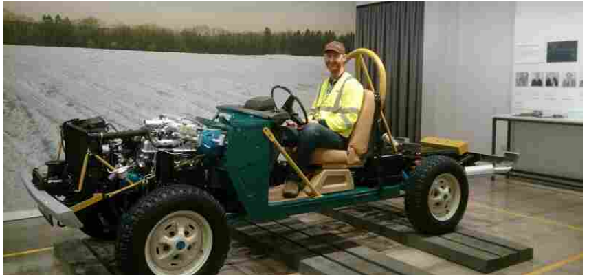
The fully driveable 1970 cutaway Range Rover engineering model designed to show the inner workings.
