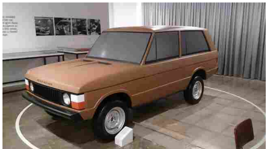
The full size clay replica showing two different styling proposals for the 1970 Range Rover
