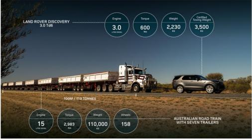
with the rolling resistance of so many axles to overcome, is a huge achievement. We expected the vehicle to do well but it passed this test with flying colours, hitting 44km/h along its 16km route."
