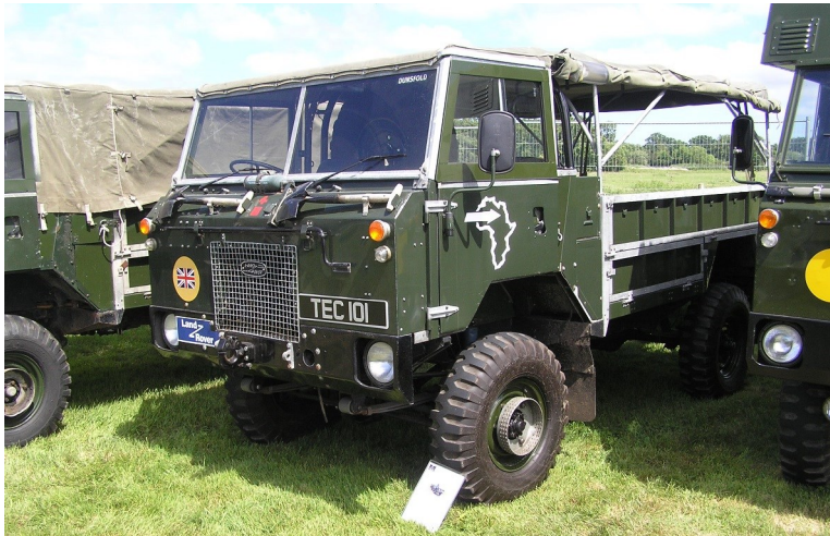
1974 101" Forward Control Trans-Sahara Expedition vehicle Chassis number: 95600024A Registration number: TEC 101 / 76 FL 66 Engine type: 3.5 V8 Petrol Gearbox type: 4 Speed manual Vehicle spec:
