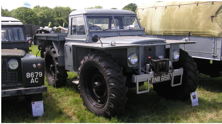
1964 Series 11A Forest Rover by Roadless Traction, Hounslow Chassis number: 25201678A Registration number: BNB 615B Engine type: 2.25 Petrol Gearbox type: 4 Speed Vehicle spec:
