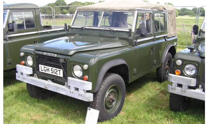
1978 Prototype Land Rover 100" for French and Swiss army evaluation Chassis number: 100S2M10X Registration number: LGH 512T Engine type: 2.25 Petrol Gearbox type: 5 Speed Vehicle spec:
