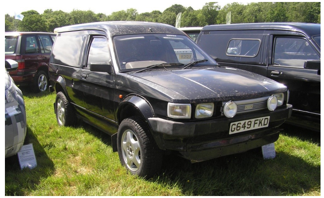
1994 Freelander test mule with Maestro van body Chassis number: SPLLNAAA7SAXXXX09 Registration number: G649 FKO Engine type: 1.8 ohv Petrol Gearbox type: 5 Speed Vehicle spec:
