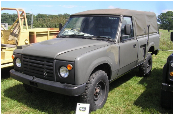
1991 Challenger Prototype Chassis number: JUNO01 Registration number: None Engine type: 2.5 Gem 2 TDi Gearbox type: 4 Speed Vehicle spec: This is one of three Challenger Prototypes built in 1991. The idea was to have a common platform for all vehicles in the Land Rover model range. The chassis and cab are based on the Discovery 1 and the body is hand made to fit the 114" chassis. The vehicle was the only military-style pick-up made although it is really only a mock-up and never intended to be driven – even the sills are made of wood! The other two were civilian station wagons. On this vehicle the door tops and windscreen are removable to create a low silhouette vehicle. The engine is a prototype of the 300TDi Gemini 2 (although the air cleaner was never made) and the gearbox is a Range Rover 4 speed automatic. The axles are Discovery to Camel Trophy specification. Electrics are 12V and 24V. This is the only surviving Challenger – the other two were crushed.
