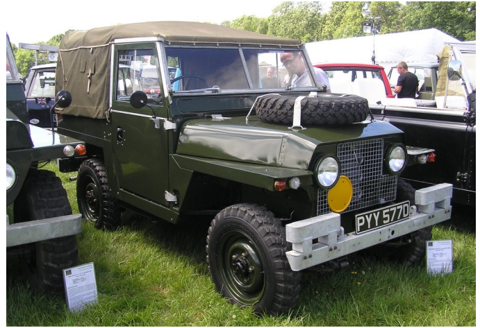
1966 Prototype Half Ton 'Lightweight' military evaluation vehicle Chassis number: 24125945 Registration number: PYY 577D / 21 BT 85 Engine type: 2.25 Petrol Gearbox type: 4 Speed Vehicle spec: This is one of the first prototypes of the Half Ton 'Lightweight Land Rover. It is one of six built in 1966 for MoD evaluation and all were extensively modified as the trials progressed. Our vehicle initially carried the service number 00 SP 15 and then 21 BT 85. It was sold at the MoD sale at Ruddington in August 1983 and was later painted blue. Somewhat used and abused, it came up for sale on an internet auction site in 2008 and was acquired by us. There is very little on the body or chassis that is similar to the eventual production models. The chassis and bulkhead required extensive restoration caused, we think, by wading and sea trails early in its military career but we were able to save and re-use the body panels. We think this is probably the oldest Half Ton on the road today.
