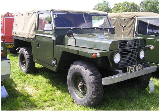
1966 Land Rover 110" Air-portable Gun Tractor Prototype Chassis number: 110-1 Registration number: VXC 100F Engine type: 3.0 6cyl Petrol Gearbox type: 5 Speed Vehicle spec: This odd prototype was one of three built as a private venture by Rover as an air-portable gun tractor. It was also designed to tow a power-driven trailer with the 105mm Field Gun behind that – a Rover take on the old Morris 'Quad' which towed an ammunition limber and the 25-pound gun. These prototypes were in Rover military engineering at the same time as the 88" Half Ton and the 101" Forward Control. The MoD eventually awarded a contract to Land Rover but it was for the 101" Forward Control rather than for this vehicle, and the project for the 110 Gun Tractor was eventually stopped in 1968. This is the first of the three and differs slightly from the only other survivor which is number two. The gearbox is a Turner 5 speed and it has two transfer boxes to enable trailer drive in low box. We acquired our vehicle from Land Rover in 1972 where it had been in use as a gang mower. We drove it home and from that day on we consider it to be by far the worst Land Rover to drive of any we have experienced. A full restoration was carried out in 1994.
