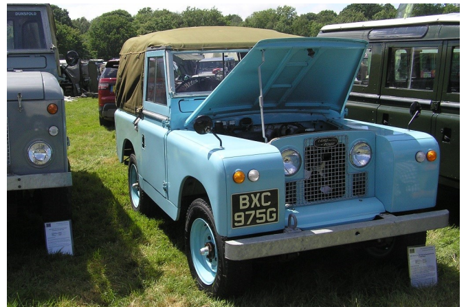
1967 Series 11A 88" Buick V8 test-bed for the Range Rover Chassis number: 8884/2158 Registration number: BXC 975G Engine type: 3.5 V8 Petrol Gearbox type: 4 Speed. Vehicle spec: This 88" is totally unique. It has a prototype V8 Buick engine fitted by Land Rover in 1967. The registration number is later than the vehicle build date as it ran around on trade plates prior to registration. It is one of three test-beds built for mileage testing with the V8 prior to its installation in the new Range Rover. It still retains the Series 11A crash gearbox but uses high-ratio differentials. It has larger brakes all round and radial tyres for high speed safety. After its trial days were over it went to the test track at Gaydon where it towed a surface friction trailer for many years. At this stage it was fitted with a station wagon hard top and was painted Masai Red with the roof painted in Sahara Dust, which was apparently a paint scheme trial. Since acquiring it, we have completed a ground-up restoration and decided to finish the vehicle as it was in the late 1960s. The light blue was never a Land Rover production colour but the three test vehicles were all paint assessment cars as well. The other two cars were broken up, making this the sole survivor of the vehicles that played an important role in the development of the Range Rover.
